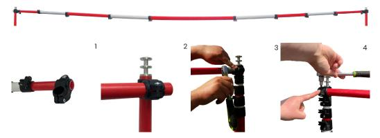
Position the crossbar elbow for placement onto the GS6 pole. Then slide the crossbar down onto the GS6 pole, fully over the steel end top section (like in image 2). To finsh, secure the crossbar by tightening the elbow with an allen key fitting. Ensure this has been completed on both elbows.
